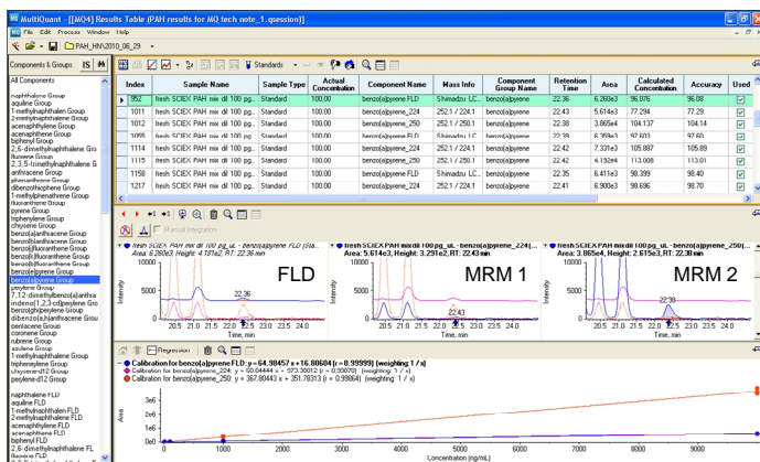
Figure 8. Quantitation of Benzo(a)pyrene using FLD (left) and MRM mode (middle and right)
